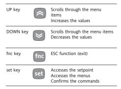
At start-up the instrument performs a Lamp Test; for few seconds the display and the leds blink, in order to verify their integrity and correct operation. The instrument has two main menus: the "Machine Status" and "Programming" menu.
